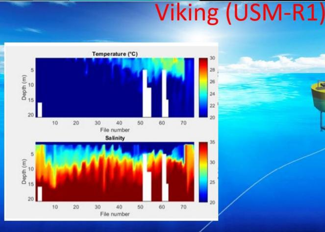
Viking: The oceanographic and meteorological buoy equipped with a automatic CTD profiler. Meteorological parameters
